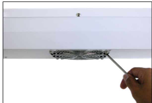
Figure 10. Shorting the ionizer's two fan grills
