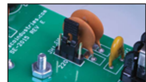
Figure 8. 220 VAC jumper setting
